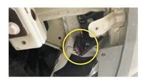
**9.** Remove the bumper by carefully unclipping starting on the left corner, moving away from the headlight.
